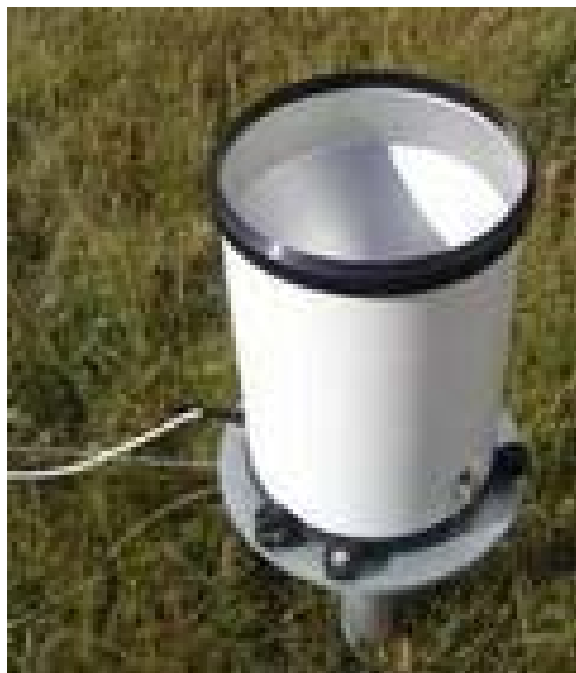
tipping bucket Pluviometer with a heating
